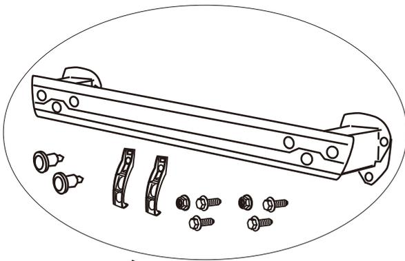
Discard bumper beam and hardware shown. These items will not be re-installed.
