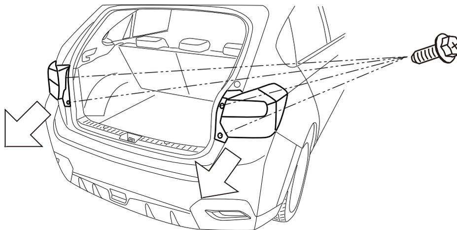
Remove bolts from tail light housings and carefully pull back on tail light housings to remove. Unplug connectors.
