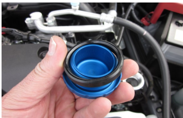
3: INSTALL GASKET IN SPT OIL CAP
