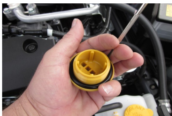
2: USE SCREWDRIVER TO REMOVE GASKET
