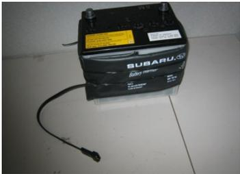
6 Place the battery back in the vehicle. Tighten battery hold down bolts taking care not to pinch the warmer. Reconnect the positive terminal first followed by the negative terminal.
